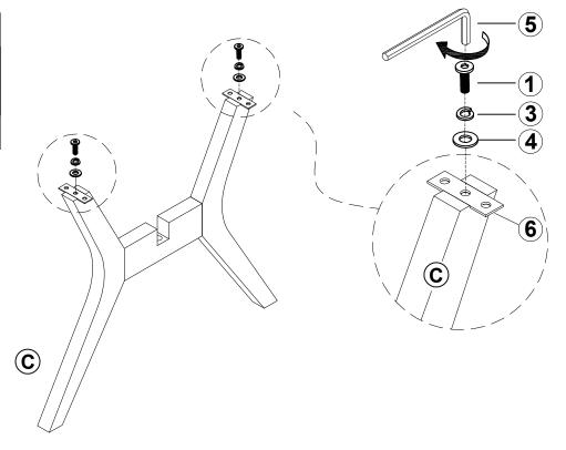
Attach connector (6) to leg frame (C) with bolt (1) and flat washer(4) and spring washer(3), tighten it with Allen wrench (5).
