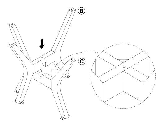
Attach the leg frame (B) to leg frame (C) by align the slot .
