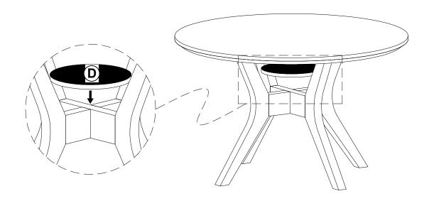
Attach the Shelf Panel (D) to the middle of the unit pre-assembled on step 6 by hand. now your table is ready for use .
