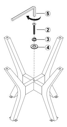
Use bolt (2) and spring washer (2) and flat washer (3) and Allen Wrench (5) to tighten, As shown.
