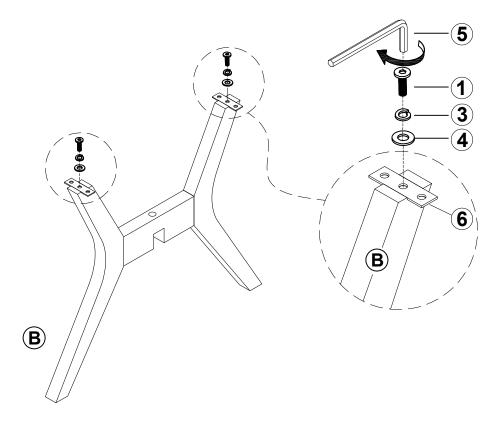
Attach connector (6) to leg frame (B) with bolt (1) and flat washer(4) and spring washer(3), tighten it with Allen wrench (5).
