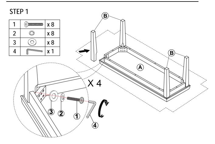
Attach the Leg (B) to Seat Frame(A), use the Bolt (1), Spring Washer(2) and Flat Washer(3), tight Bolt (1) with Allen Wrench (4) as shown.
