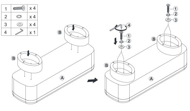
Note : Fully tighten the bolts in sequence after all bolts proper connected. STEP 3
