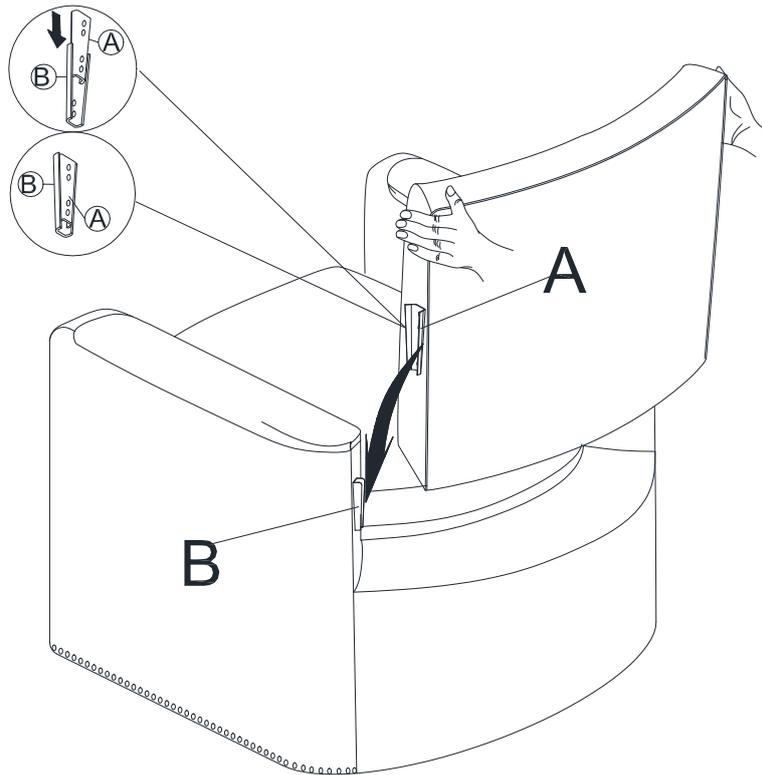
Attach the back (A) to the seat (B) as shown. Make sure the male and female brackets align as shown.
