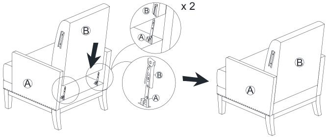
Attach the Back (B) to the seat frame (A) by sliding the receivers into the mechanism posts located on the seat frame (A).
