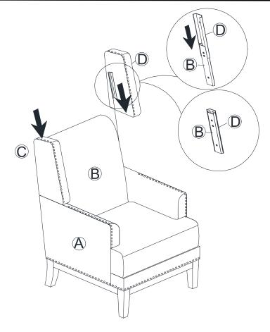
Attach the back wing (C) (D) to the back as shown. Make sure the male and female brackets align as shown.
