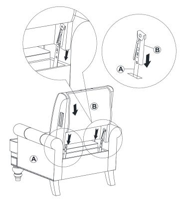
Attach the Back (B) to the Seat (A) by sliding the receivers into the mechanism posts located on the Seat (A).
