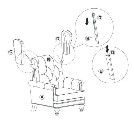
Attach the back wing (C) (D) to the back as shown. Make sure the male and female brackets align as shown.
