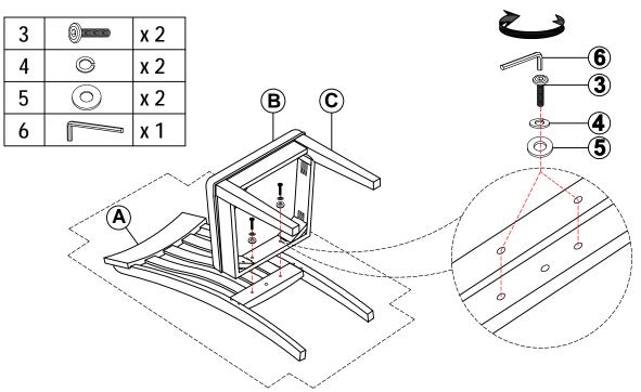
Attach the Seat Frame (B) to Chair Back (A), use the Bolt (3), Spring Washer(4) and Flat Washer(5), tight Bolt (3) by Allen Wrench (6).
