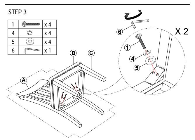
Use Bolt (1), Spring Washer (4) and Flat Washer (5), tight Bolt (1) with Allen Wrench (6) as shown.
