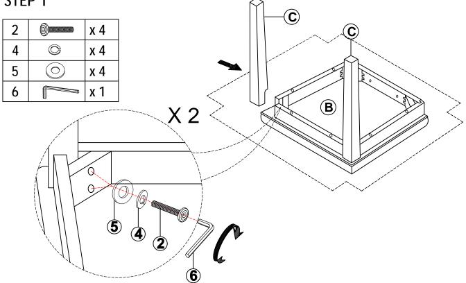
Attach the Front Leg (C) to Seat Frame (B), use the Bolt (2), Spring Washer(4) and Flat Washer(5), tight Bolt (2) with Allen Wrench (6) as shown. ( Don't tighten bolt until at step 3)
