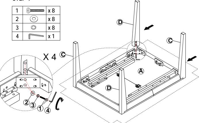
Attach the Leg (C) (D) to Table Top (A), use the Bolt (1), Spring Washer(3) and Flat Washer(2), tight Bolt (1)with Allen Wrench (4) as shown.
