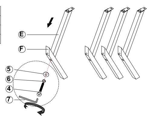
Attach Wood Support Top(E) to Wood Support Bottom (F), use the Bolt (4), Spring Washer(6) and Flat Washer(5), tight Bolt (4) with Allen Wrench (7) as shown.
