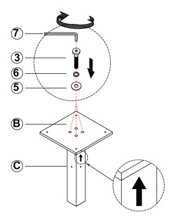
Attach Connect Panel (B) to Poster (C), use the Bolt (3), Spring Washer(6) and Flat Washer(5), tight Bolt (3) with Allen Wrench (7) as shown.
