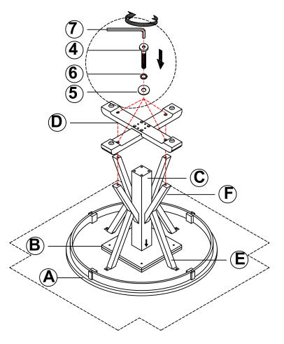
Attach Base(D) to Wood Poster (C) , use the Bolt (4), Spring Washer(6) and Flat Washer(5), tight Bolt (4) with Allen Wrench (7) as shown.
