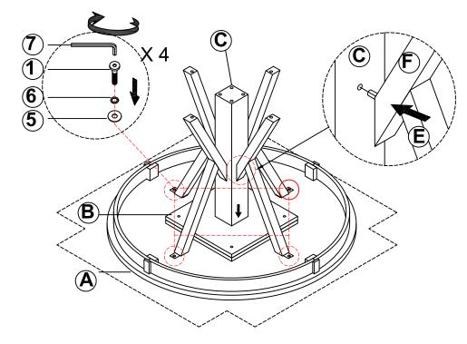
Attach Wood Support Top(E) and Wood Support Bottom (F) to Table Top (A), Use the Bolt (1), Spring Washer(6) and Flat Washer(5), tight Bolt (1) with Allen Wrench (7) as shown.
