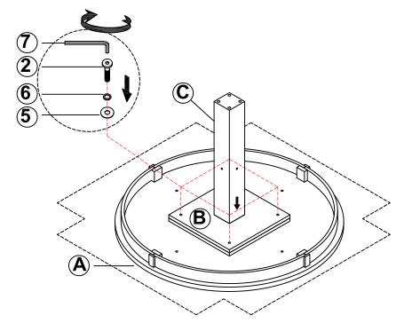
Attach Connect Panel (B) and Wood Poster (C) to Table top (A), use the Bolt(2), Spring Washer(6) and Flat Washer(5), tight Bolt(2) with Allen Wrench (7) as shown.
