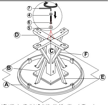
Use the Bolt (4), Spring Washer(6) and Flat Washer(5), tight Bolt (4) with Allen Wrench (7) as shown.
