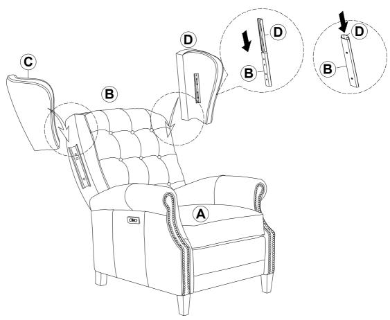
Attach the back wing (C) (D) to the back. Make sure the male and female brackets align as shown.
