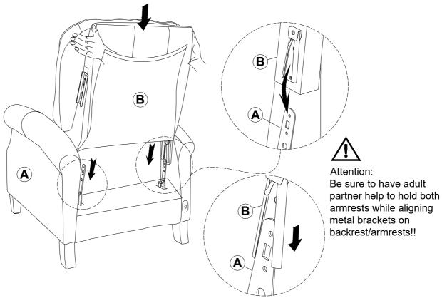
Attach the Back (B) to the Seat Frame (A) by sliding the receivers into the mechanism posts located on the Seat Frame (A).
