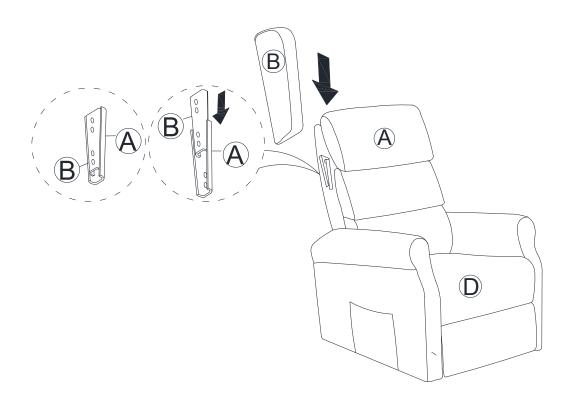
receivers into the mechanism posts located on the seatframe (D).
