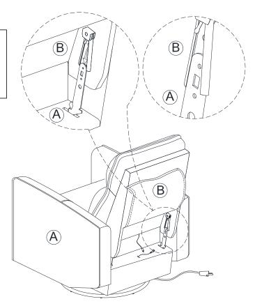
Attach the back (A) to the seat (B) as shown. Make sure the male and female brackets align as shown.
