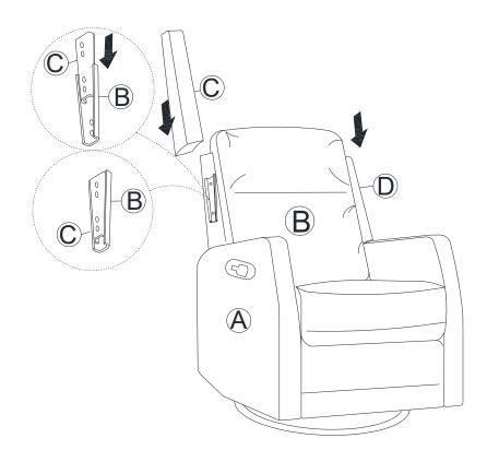
Attach the back wing (C) (D) to the back . Make sure the male and female brackets align as shown.
