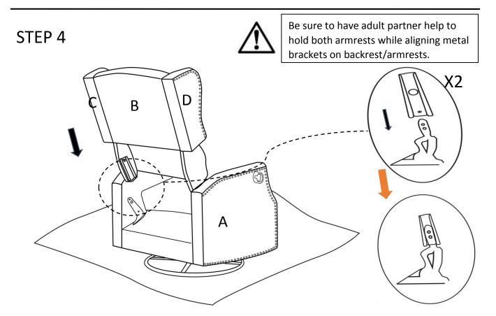
Insert the small metal arms on the sides of the Chair Backrest(B) into the prefabricated slide lock gadget on the Chair Base(A) as shown above. Firmly but gently, push the Chair Backrest(B) downwards until the Backrest is fully slotted and locked into position.
