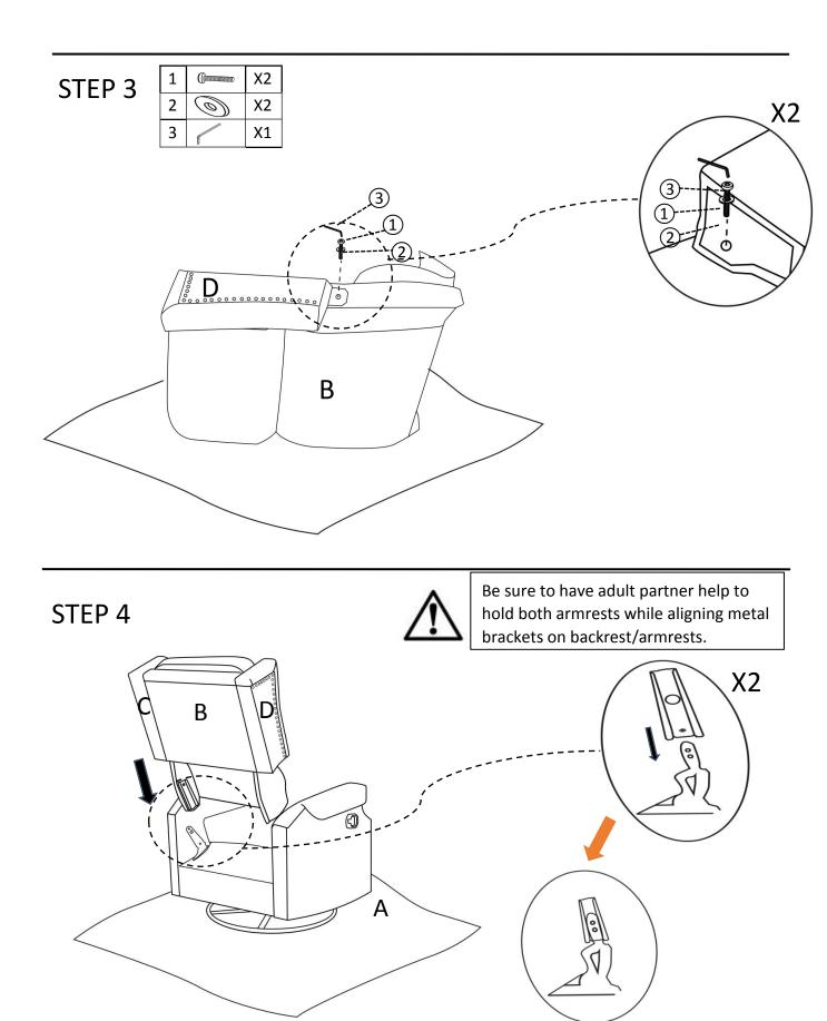
Insert the small metal arms on the sides of the Chair Backrest(B) into the prefabricated slide lock gadget on the Chair Base(A) as shown above. Firmly but gently, push the Chair Backrest(B) downwards until the Backrest is fully slotted and locked into position.
