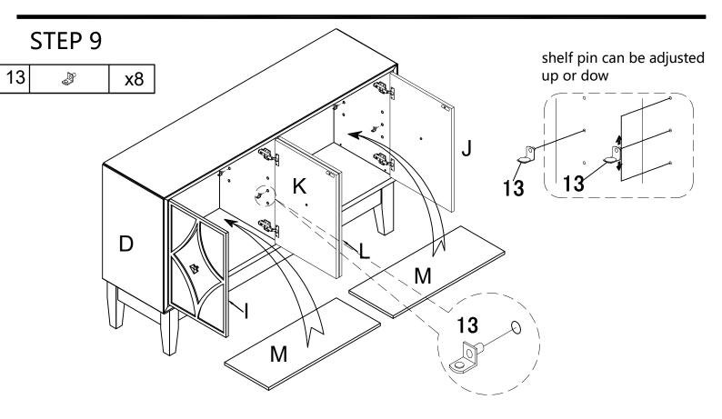
Insert shelf pin (13) to pre-assembled unit at step 8, and attach adjustable shelf (M) to it
