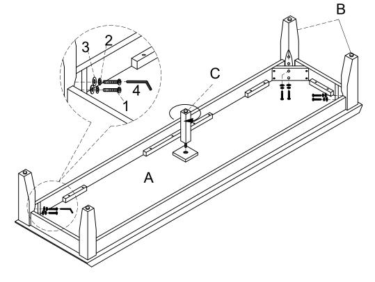
Attach leg(B/C) to bottom panel(A) with bolt(1) and flat washer(3) and spring washer(2), tight it with Allen wrench(4).
