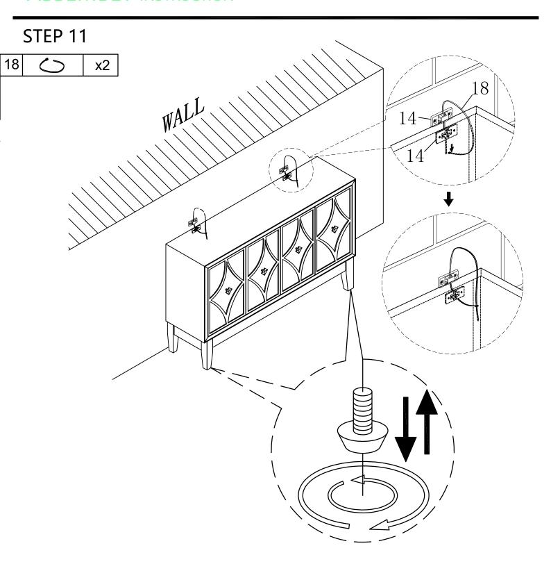
Attach the unit to the wall with tie(18)
