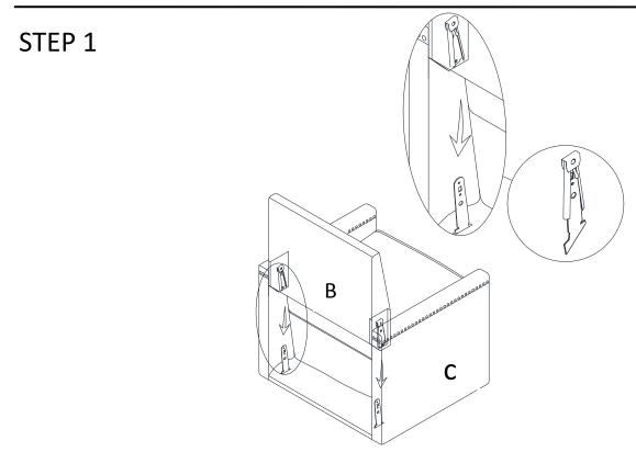
Attach the back frame (B) to the seat (C) as shown. Make sure the male and female brackets align as shown.
