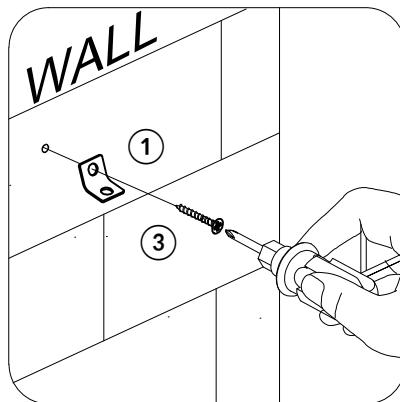
2. Secure the Anti-tip device ① to the wall with screws ③
