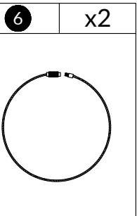
insert the metal cable of part 6 through the holes of part 7 and tighten the two threaded ends firmly together.
