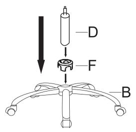
**STEP 2:**Attach the metal cover F on top of the spider base B then insert the gas lift D to the center hole of the base B.
