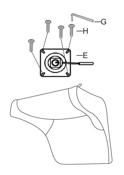
**STEP 3**: Use bolt H and allen key G to attach mechanism E to bottom of the seat cushion A,make sure the holes on under seat align with metal plate, then fasten bolts to secure.
