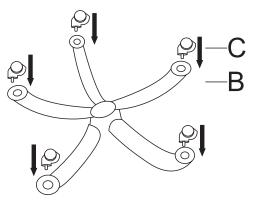
**STEP 1**:Insert casters C to bottom of the spider base B.
