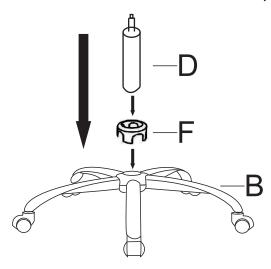
**STEP 2:**Attach the metal cover F on top of the spider base B then insert the gas lift D to the center hole of the base B.
