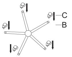
**STEP 1**:Insert casters C to bottom of the spider base B.
