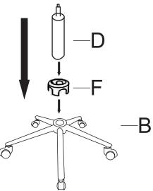
**STEP 2:**Attach the metal cover F on top of the spider base B then insert the gas lift D to the center hole of the base B.
