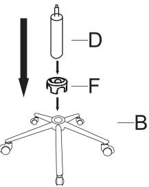
**STEP 2:**Attach the metal cover F on top of the spider base B then insert the gas lift D to the center hole of the base B.
