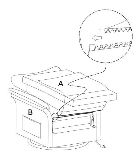
Hold both armrests while aligning metal brackets on backrest or armrests.
