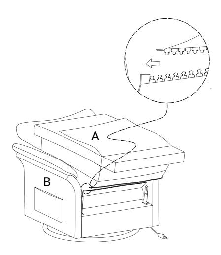
Hold both armrests while aligning metal brackets on backrest or armrests.
