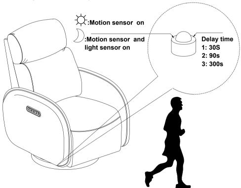
Place sensor directly to motion range of people light will on when detect motion, light off when there is no motion detected within a delay time.
