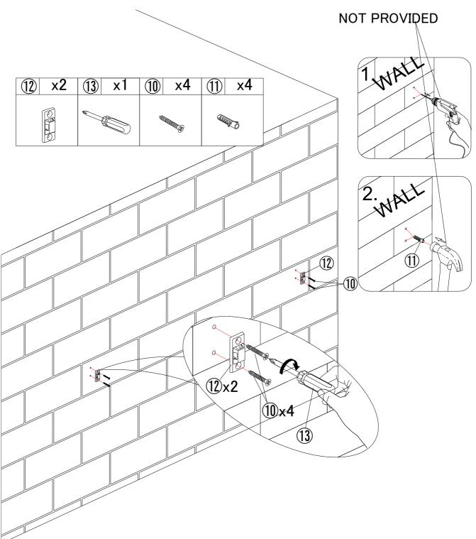
STEP17:Install the anti-collapse device.
