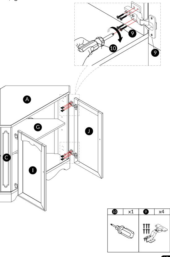
Use screw #1 to attach middle door (I & J) pre-assemble unit at step 9 ,tighten screw #1 with screwdriver #10 .
