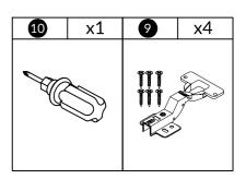
Use screw #9 to attach left door (I) and right door (J) to pre-assemble unit at step 8 ,tighten screw #9 with screwdriver #10 .
