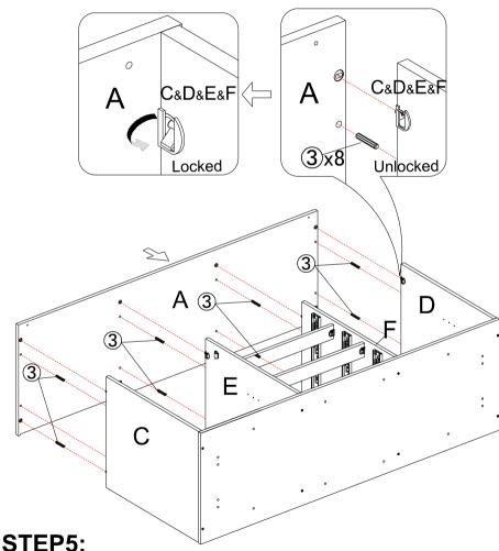
Insert wooden dowel ③ into preassembled unit at step 4, and then insert top panel (A) into preassembled unit at step 4, make sure all holes aligned and pull the combiner to lock it.
