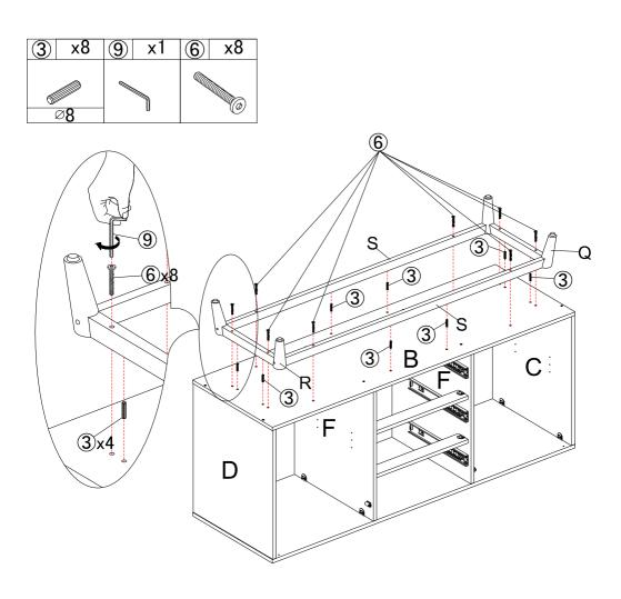
**STEP8:**Insert wooden dowel ③ into the corresponding hole of bottom panel(B),and then insert preassembled step 6 into bottom panel (B),use bolt ⑥ to attach them , tighten bolt with allen key ⑨.
