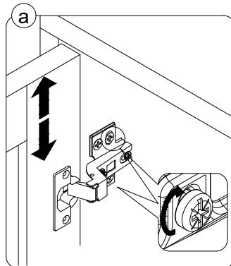
To adjust the door vertically loosen the screw as shown and move up and down as needed.
