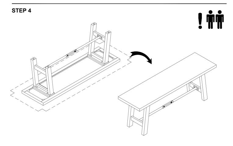
Flip the assembled bench over to complete the assembly.
