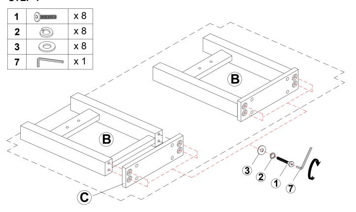
Use Bolt(1), spring washers (2), and flat washers (3) to assemble the legs and the Connecting Plate (C) together.
