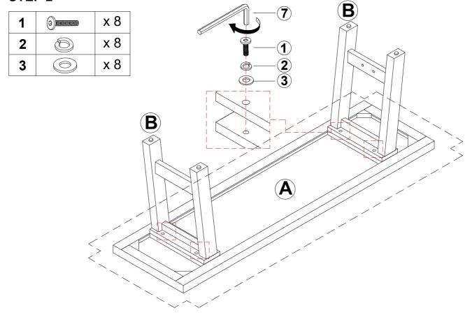
Use Bolt(1), spring washers (2), and flat washers (3) to assemble the leg frame to the bottom of the bench panel.
