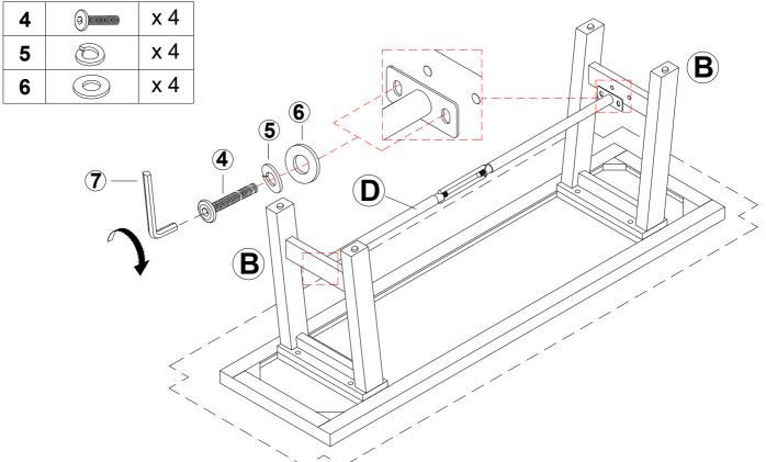
Use Bolt(4), spring washers (5), and flat washers (6) to assemble the metal connecting rod (D) between the two leg frames.
