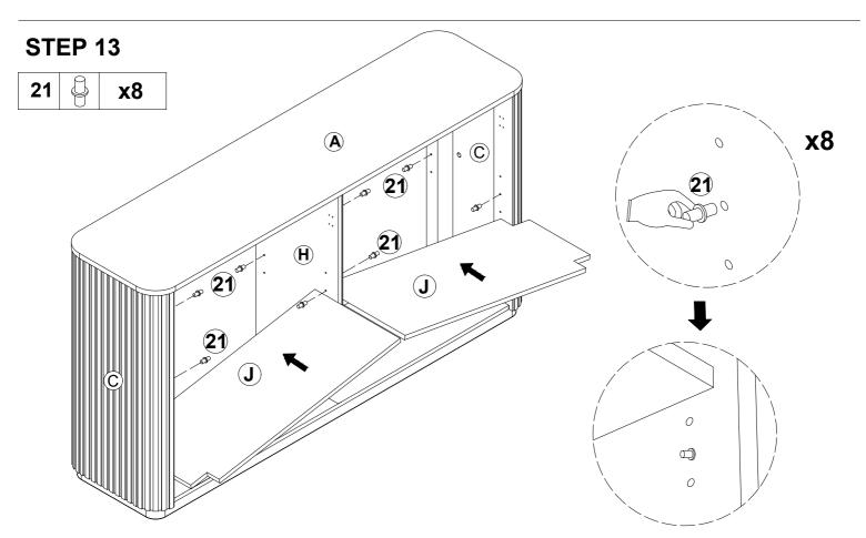
Insert shelf support (21) into the hole of inside pre-assembled cabinet and then tilt the adjustable shelf(J) and place it on the shelf support (21)
