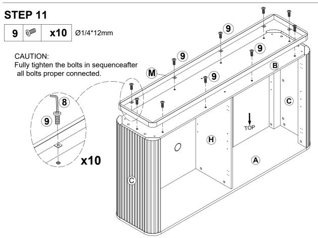
Attached metal frame (M) to the pre-assembled frame, Then insert the bolt (9) into the hole of metal frame (M) and tighten it with a allen wrench(8) as shown
