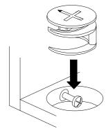
Quickfit head should be in the centre of the cam lock when the two panels are joined.
