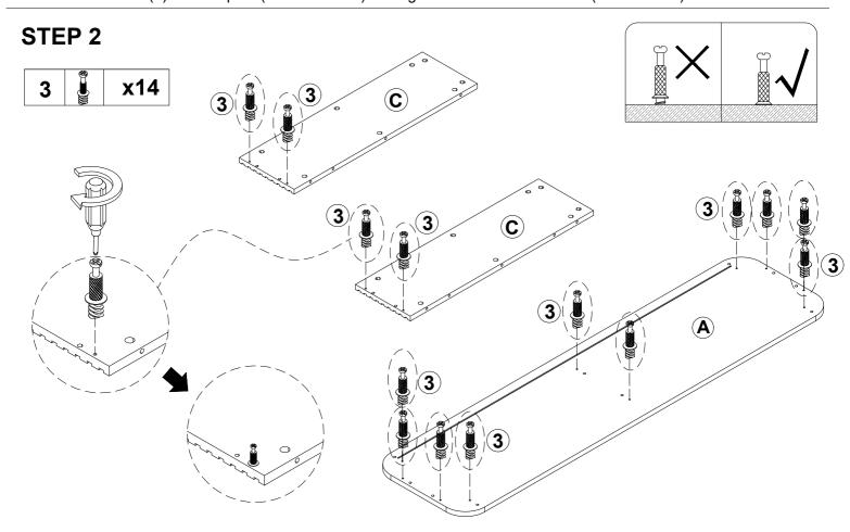
Insert the cam bolts (3) into the top panel (A) ,side panel (C) and tighten it with a screwdriver (not included) as shown.
