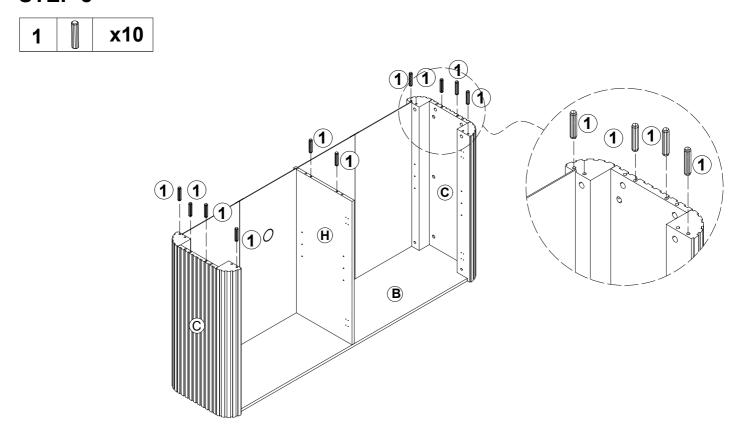
1. Insert the wood dowel(1) into the hole of pre-assembled frame top as shown .
