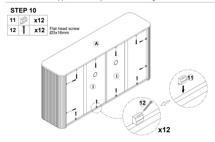
Insert plastic wedge(11) into the gap at the edge of the back panel (I) and then insert the flat head screw (12) into the hole of the plastic wedge(11) tighten it with a screwdriver as shown.
