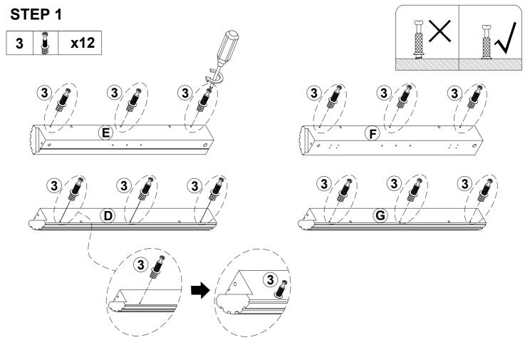
Insert the cam bolts (3) into the post (D &E & F & G) and tighten it with a screwdriver (not included) as shown.
