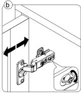
To adjust the gap from the door to the main frame turn the screw clockwiseoranti -clockwiseas needed.
