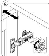
To adjust the door laterally adjust the screw as shown by turning clockwiseor anti-clockwise.
