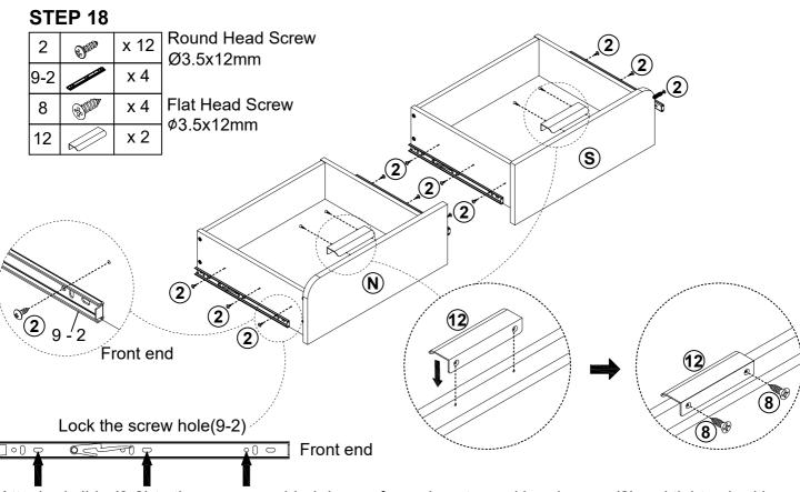
Attached slide (9-2) to the pre-assembled drawer frame, Insert round head screw (2) and tighten it with a screwdriver, Attached handle (12) to the drawer front panel, insert flat head screw(8) into hole of handle (12) tighten it with a screwdriver as shown.
