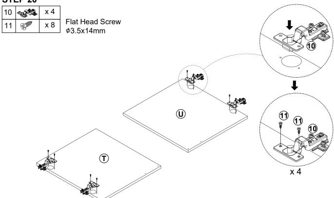
Insert hinge (10) into the hole of the door (T&U), Use screw (11) with tighten a screwdriver as shown.
