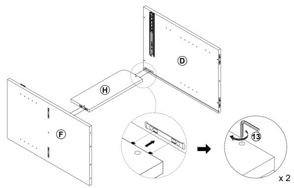
Insert the back right panel(H) into the hole of middle right vertical panel(F)/right side panel (D) and tightenit with a Allen wrench(13)as shown.
