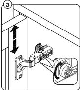
To adjust the door vertically loosen the screw asshown and move up and down as needed.
