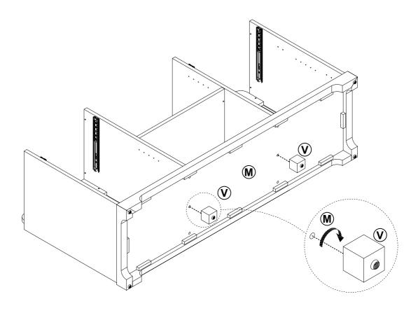
Attached part (V) to the part(M) with tighten it as shown.
