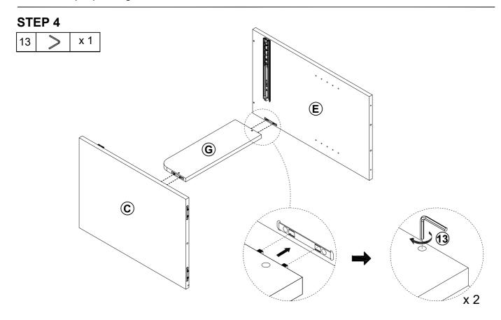
Insert the back left panel(G) into the hole of middle left vertical panel(E) / left side panel (C) and tighten it with a Allen wrench(13) as shown.
