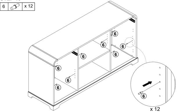
1.Insert the support shelf (6) into the hole of the pre-assembled cabinet as shown.
