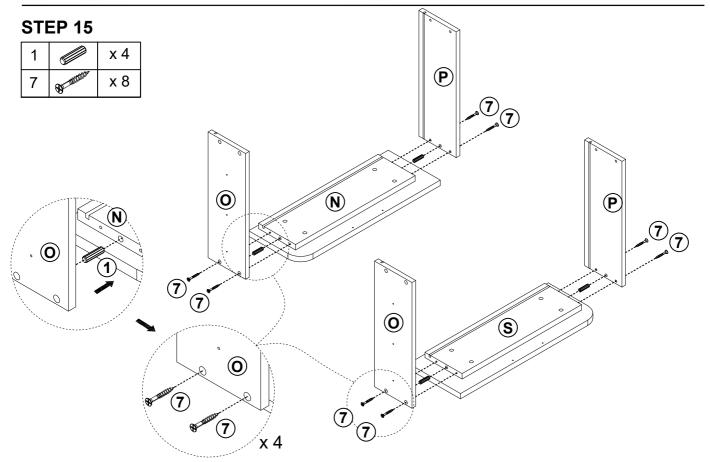
Insert the wood dowel  $\ (1)$  into the hole of the drawer front panel  $\ (N\&S)$  to connect the drawer side panel  $\ (O\&P)$ , Use screwdriver to tighten screw  $\ (7)$  as shown.
