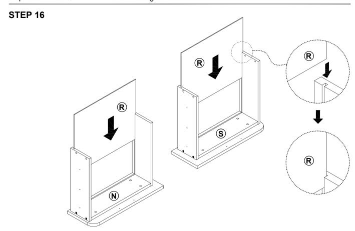
Insert drawer bottom panel (R) into the solt of pre-assembled drawer frame(N&S) as shown.
