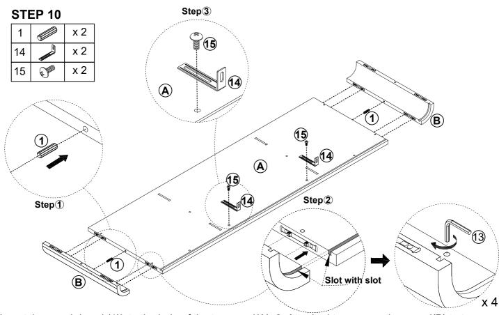
1.Insert the wood dowel (1)into the hole of the top panel(A), 2. Attached top connecting panel(B) to top panel (A), Then tighten it with a Allen wrench(13), Attached anti tipping hardware(14) to the top panel(A) and tighten it with a screwdriver as shown.
