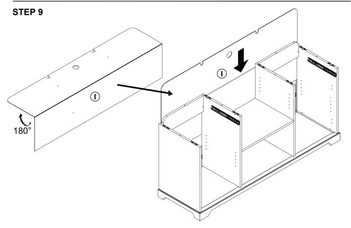
Open the folded back panel, Then align it and insert back panel(I) into the slot of pre-assembled frame as shown.
