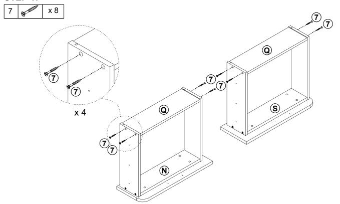
Attached drawer back (Q) to the pre-assembled drawer frame, Insert screw(7) into the hole of pre-assembled drawer frame and tighten it with a screwdriver as shown.
