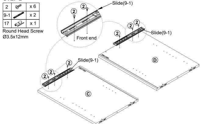
Attached slide(9-1) to left and right side panel(C&D), Then insert the round head screw(2) into the hole of slide(9-1) and tighten it with a screwdriver(17) as shown.
