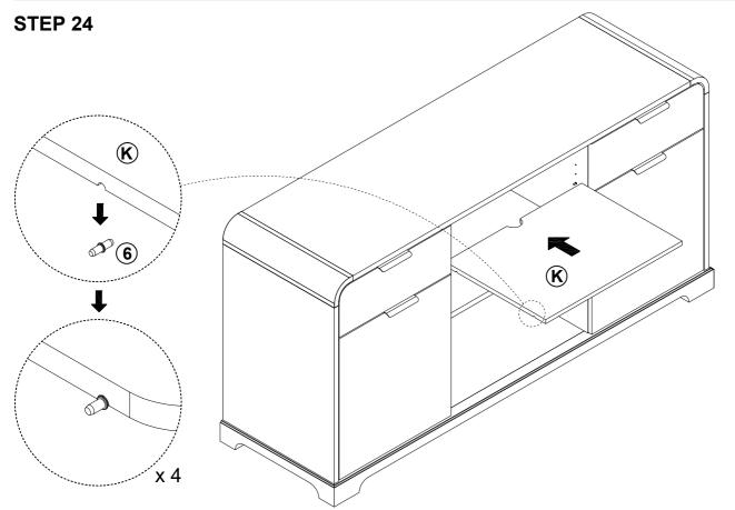
Place adjustable shelf(K) inside the cabinet, Make sure that shelf support(6) is placed in the slots of adjustable Shelf (K).
