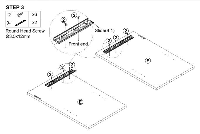
Attached slide(9-1) to left and right vertical panel(E&F), Then insert the round head screw(2) into the hole of slide(9-1) and tighten it with a screwdriver as shown.
