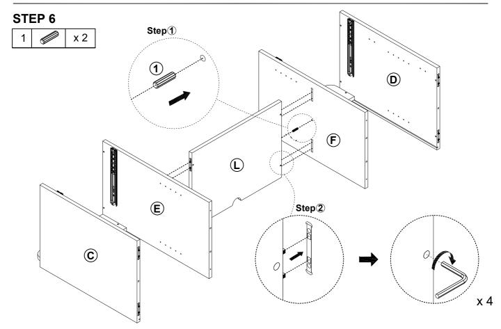
1.Insert the wood dowel (1)into the hole of the middle fixed shelf (L), 2. Insert the middle fixed shelf (L) into the hole of middle left and right vertical panel(E&F), Tighten it with a Allen wrench(13)as shown.
