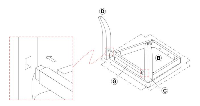
Pre-assemble the stretcher(G) into the correct holes of the legs (C) and (D).
