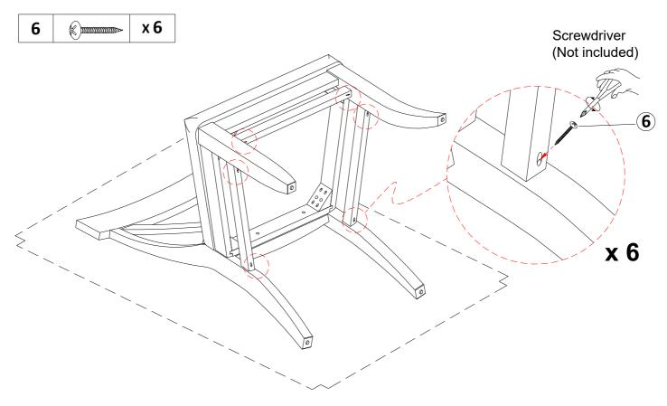
Use wood screws (6) as shown in the diagram to secure the stretchers to the chair.
