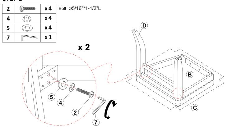
Use hardware (2), (4), and (5) to assemble the legs (C) and (D) to the seat frame (B).
