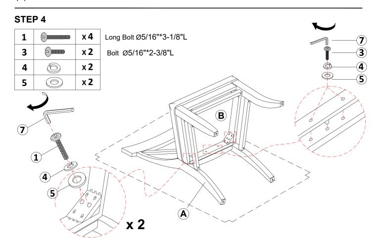
Use hardware (1), (3), (4), and (5) to assemble the seat (B) to the chair back (A).
