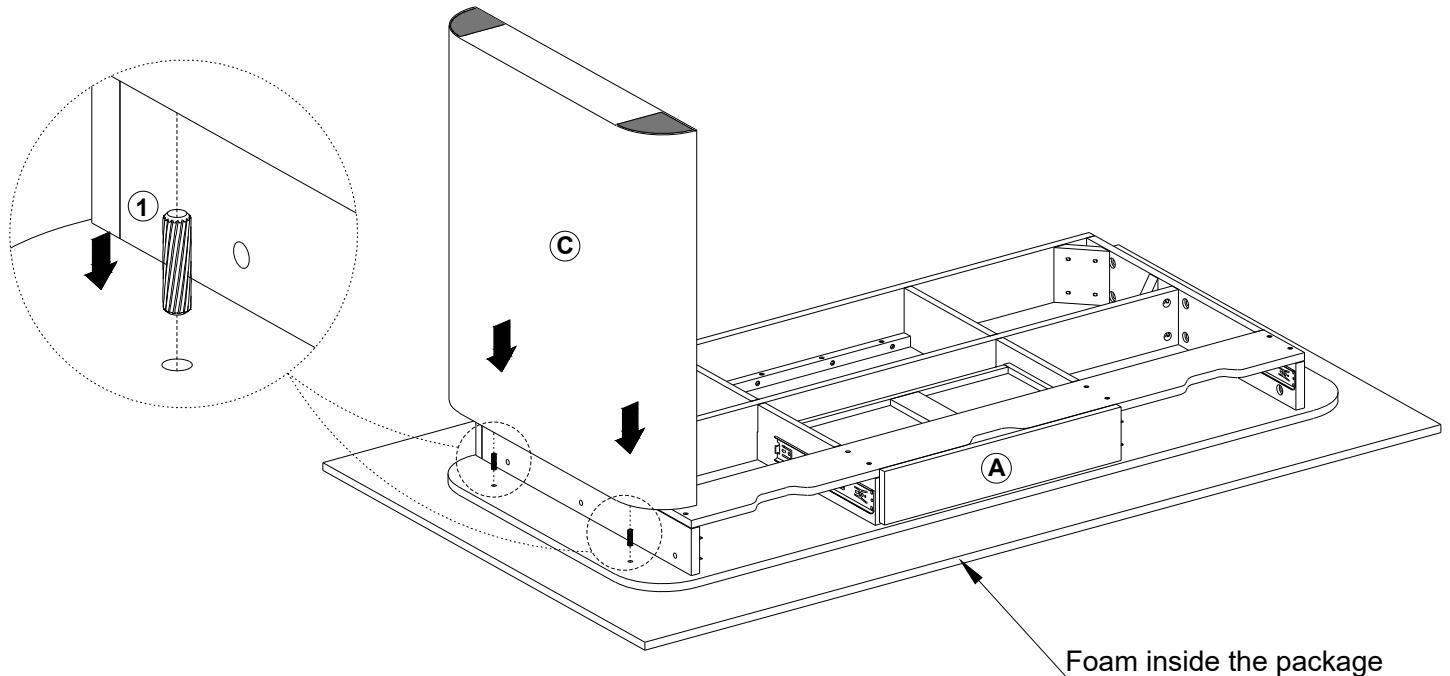
First insert wooden dowel (1) into Top panel (A), then connect left leg (C) to top panel (A).
