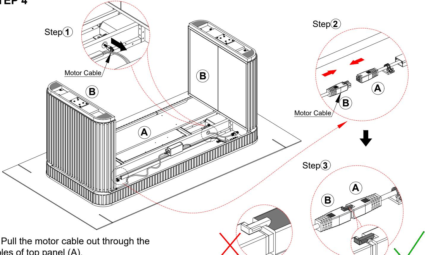
1. Pull the motor cable out through the holes of top panel (A).
