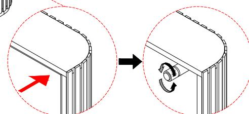
2. The doors on the foot box can be easily pushed open, and a second push will close it.
