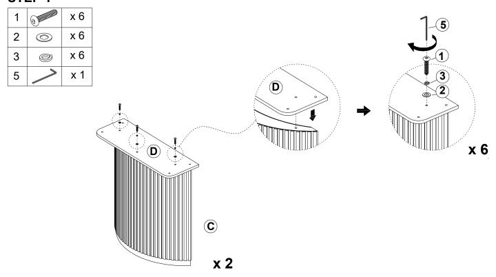
Use bolt (1) to through spring washer (3) and flat washer (2), then secure the connect panel (D) to foot (C). Fully tighten the bolt with an Allen key(5).
