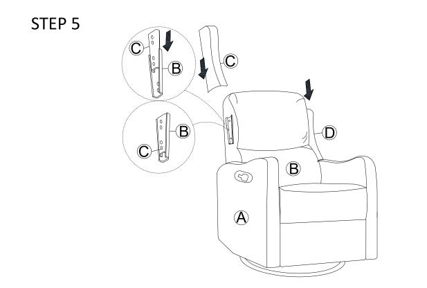
Attach the back wing (C) (D) to the back . Make sure the male and female brackets align as shown.
