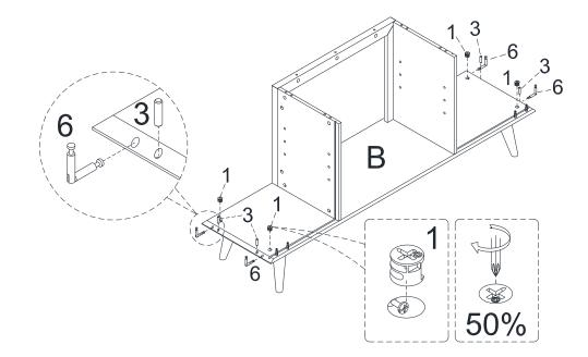
Attach Cam Bolt(6) and Cam Lock(1) and Wood Dowel(3) to Bottom Frame(B) as shown.
