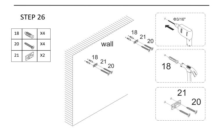
Drill hole on the wall, and insert Anchor(18), then attach Bracket(21) to it with Screw(20), tight screw with screwdriver.
