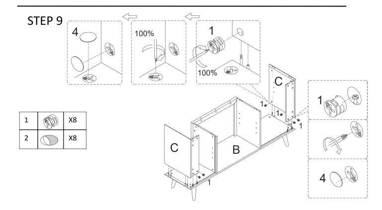
Attach Side Panel(C) to Bottom Frame(B) with Cam Lock(1) and Cover(4) ,tight it with screwdriver.
