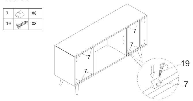
Attach Button(7) to the unit preassembly at step 17 with screw (19), and tight screw with screwdriver
