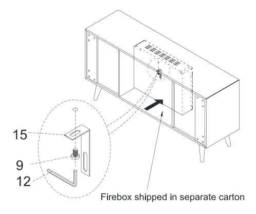
Attach Firebox to the body. with Bracket(15) and Bolt(9), tight it with Allen Wrench(12).
