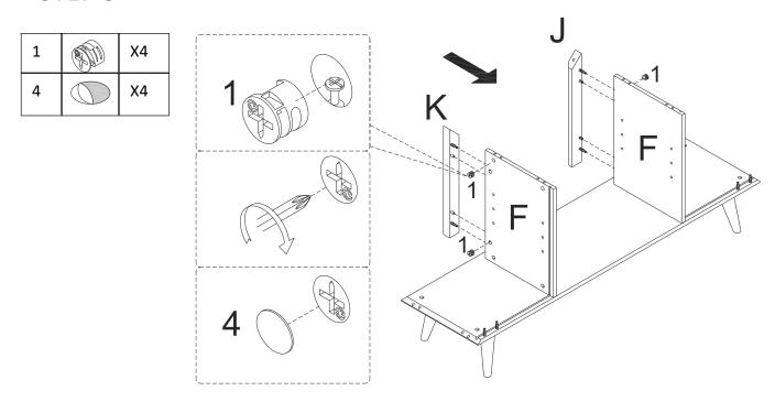
Attach Rail(J/K) to Middle Vertical Panel(F) with Cam Lock(1) and Cover(4) ,tight it with screwdriver.
