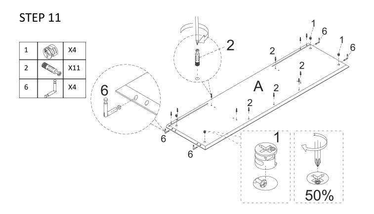
Attach Cam Bolt(2/6) and Cam Lock(1) to Top Panel(A) as shown.
