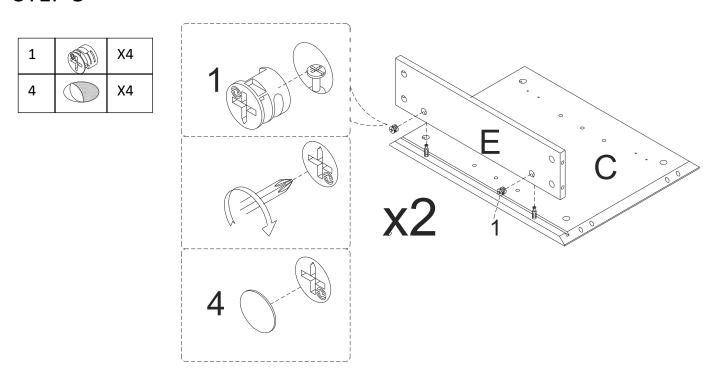
Attach Back Vertical Panel(E) to Side Panel(C) with Cam Lock(1) and Cover(4) ,tight it with screwdriver.
