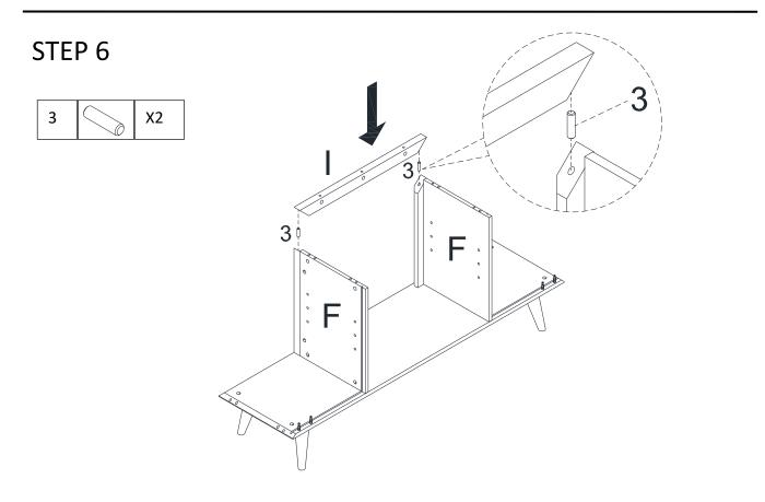
Attach Rail(I) to preassemble unit at step 5 with Wood Dowel(3) as shown.
