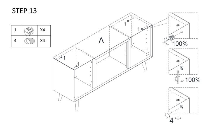
Attach cam lock (1) and cover (4) to the unit preassembly at step 12, and tight screw with screwdriver
