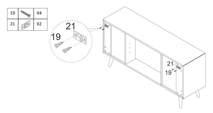
Attach Bracket(21) to the body with Screw (19), and tight screw with screwdriver
