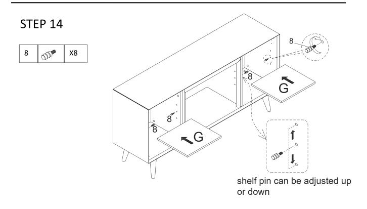
Insert Shelf Pin(8) to preassemble unit at step 13, and attach Adjustable Shelf (G) to it.
