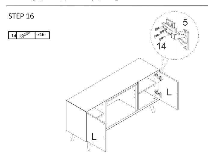
Attach Door(L) to the unit preassembly at step 14 with Screw (14), and tight screw with screwdriver
