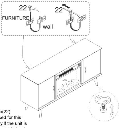
Attach the unit to the wall with Tie(22)
