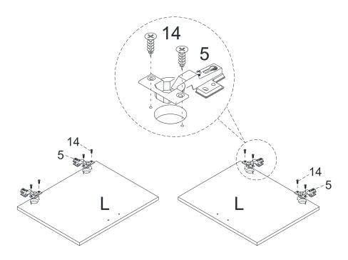
Attach Hinge(5) to Door(L) with Screw(14), then tight screw with screwdriver.
