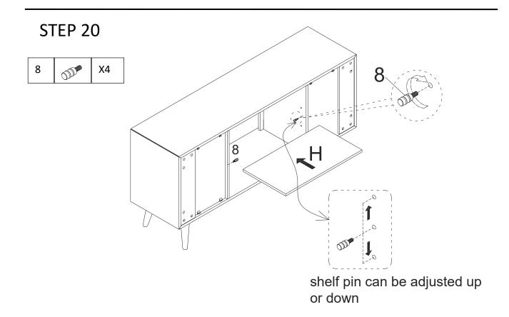
Insert Shelf Pin(8) to preassemble unit at step 19, and attach Adjustable Shelf (H) to it.
