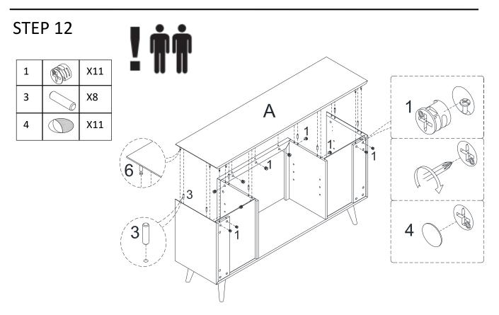
Attach Top Panel(A) to preassemble unit at step 10 with Cam Lock(1) and Cover(4) and Wood Dowel(3) ,tight it with screwdriver.
