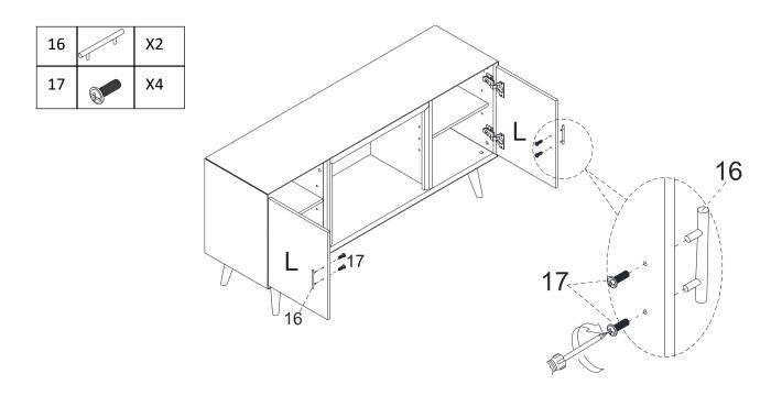
Attach Knob(16) to Door(L) with Blot (17), and tight screw with screwdriver
