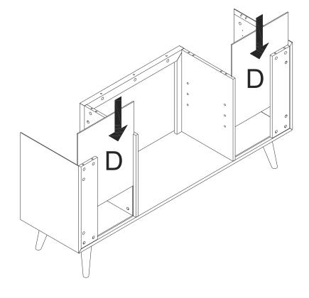
Attach Back Panel(D) to preassemble unit at step 9.
