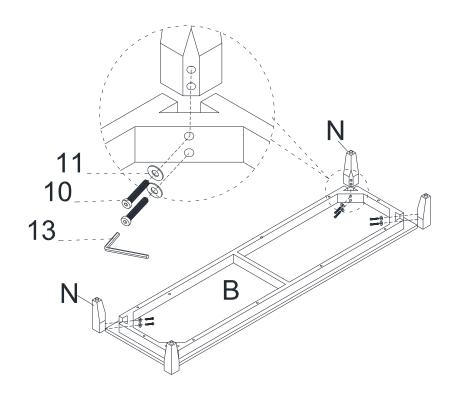
Attach Leg(N) to Bottom Frame(B) with Bolt(10) and Flat Washer(11) as shown., tight it with Allen Wrench(13).
