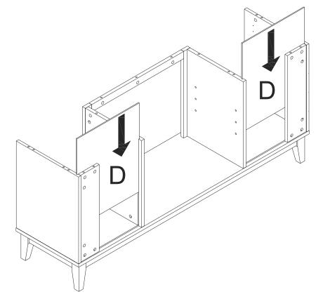
Attach Back Panel(D) to preassemble unit at step 8.
