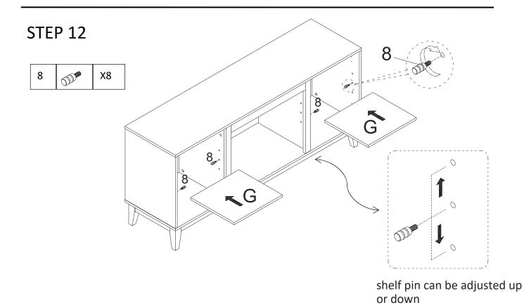
Insert Shelf Pin(8) to preassemble unit at step 11, And attach Adjustable Shelf (G) to it.
