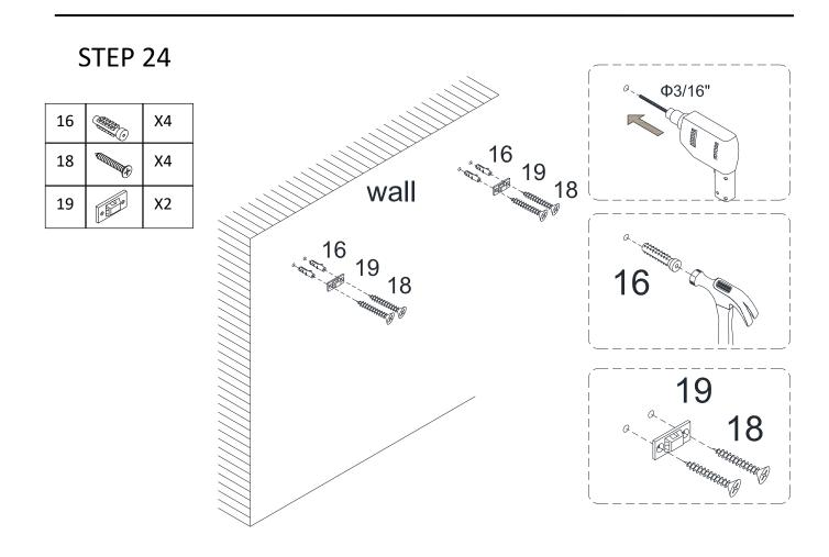
Drill hole on the wall, and insert Anchor(16), then attach Bracket(19) to it with Screw(18), tight screw with screwdriver.
