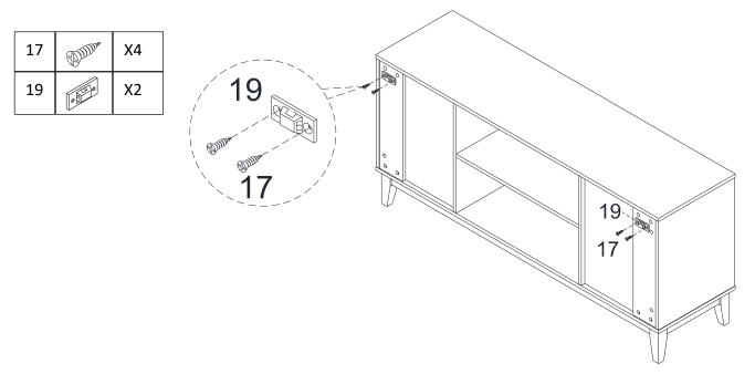
Attach Bracket(19) to the body. with Screw(17), and tight screw with screwdriver
