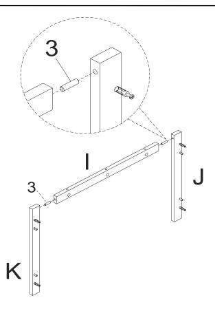
Attach Rail(J/K) to Rail(I) with Wood Dowel (3).
