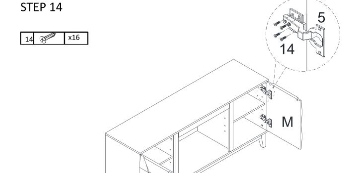
Attach Door(L/M) to the unit preassembly at step 12 with Screw(14), and tight screw with screwdriver
