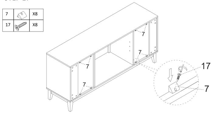
Attach Button(7) to the unit preassembly at step 16 with Screw(17), and tight screw with screwdriver
