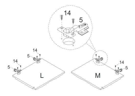
Attach Hinge(5) to Door(L/M) with Screw(14), then tight screw with screwdriver.
