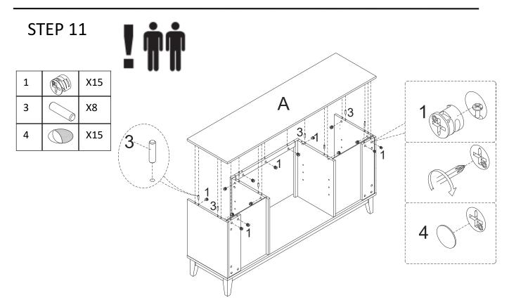
Attach Top Panel(A) to preassemble unit at step 9 with Cam Lock (1) and Cover (4) and Wood Dowel(3) ,tight it with screwdriver.
