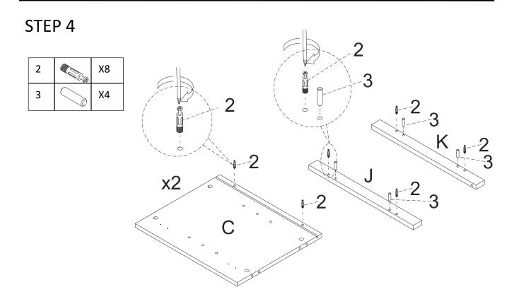
Attach Cam Bolt(2) to Side Panel(C), Attach Cam Bolt(2) and Wood Dowel(3) to Rail(J/K), tight it with screwdriver.
