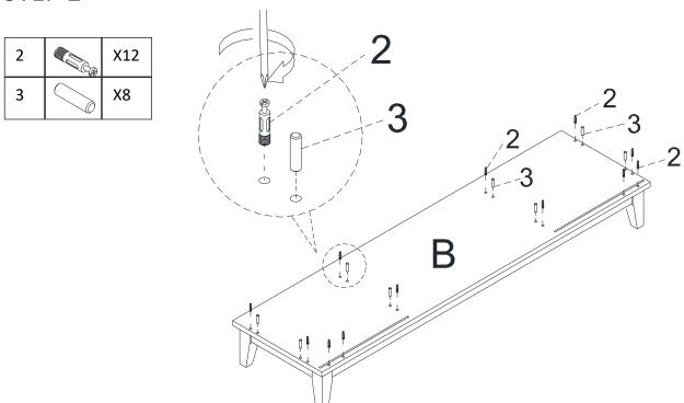
Attach Cam Bolt(2) and Wood Dowel(3) to Bottom Frame(B), tight it with screwdriver.
