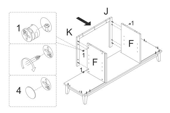
Attach Rail(J/K) to Middle Vertical Panel(F) with Cam Lock(1) and Cover(4) ,tight it with screwdriver.
