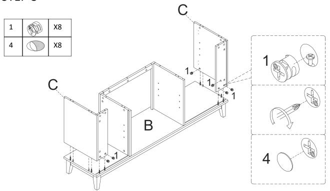
Attach Side Panel(C) to preassemble unit at step 6 with Cam Lock(1) and Cover(4) ,tight it with screwdriver.
