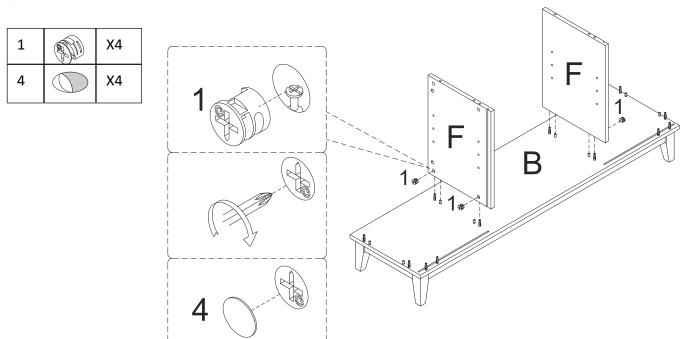
Attach Middle Vertical Panel(F) to Bottom Panel(B) with Cam Lock (1) and Cover (4) ,tight it with screwdriver.
